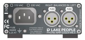
The signal inputs on the rear are equipped with XLR female type sockets, allowing balanced signal injection.
